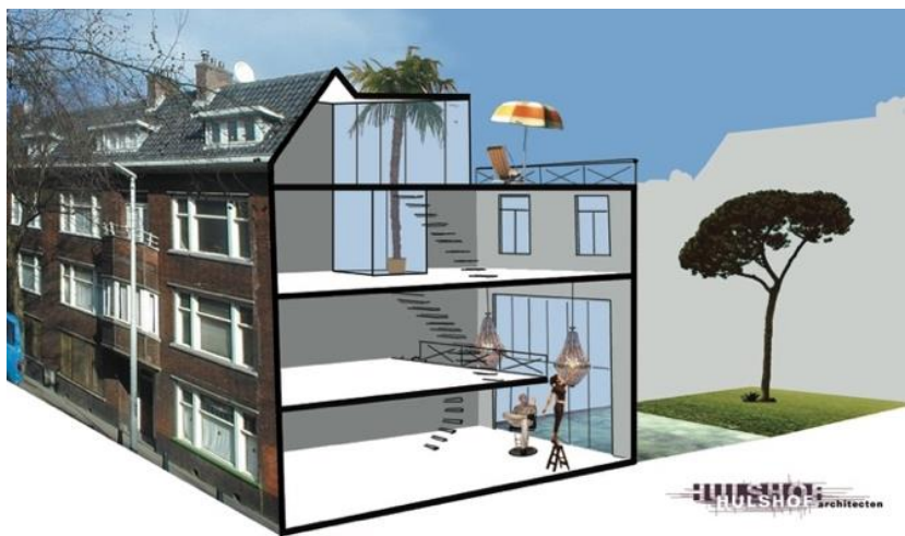
Figure 10. The Schematic Section Perspective of Renovation Showing that Front Façade and Total Height is Kept (Hulshof Architecten, 2012)
