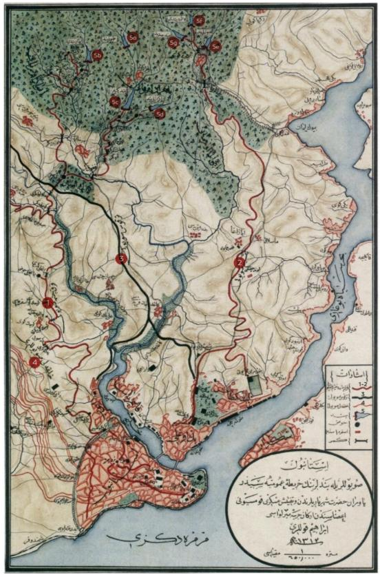
Figure 1. Map of the waterways and benders of Istanbul drawn by Mirliva Ibrahim Edhem Pasha and his son Lieutenant Nureddin Bey in the period of Sultan II. Abdülhamit [2] (1-Kırkçeşme Water System, 2-Taksim Water System, 3-Terkos Water System, 4-Halkalı Water System, 5a)Topuz Dam, 5b)Ayvad Dam, 5c)Büyük Dam, 5d)Kirazlı Dam, 5e)Topuzlu Dam, 5f)Valide Dam, 5g)II.Mahmut Dam)
