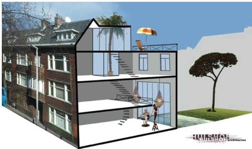
Figure 10. The Schematic Section Perspective of Renovation Showing that Front Façade and Total Height is Kept (Hulshof Architecten, 2012)
