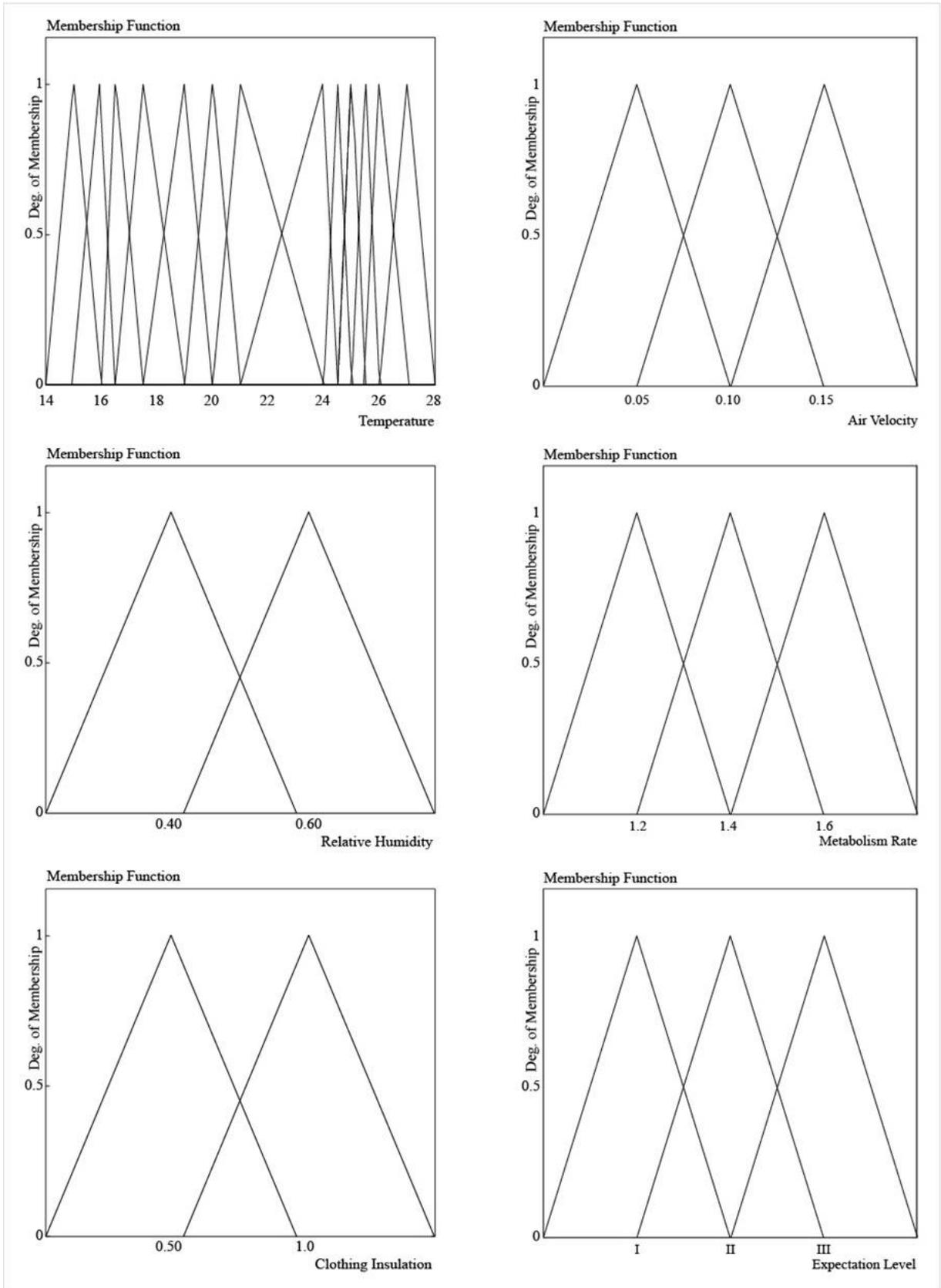
**Figure 3.** Degree of membership graphics of triangular membership functions of the inputs identified in the MATLAB program (operative air temperature, relative humidity, air velocity, metabolism rate, clothing insulation and expectation level)
