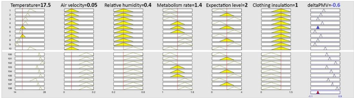
Figure 9. Rule Inference and the  $\Delta PMV$  output for Rule No. 5 ( $\Delta PMV = -0.6$ )
