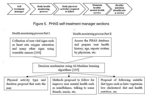
Figure 6. PHAS self-treatment manager working mechanism
