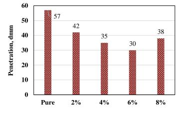
Figure 2. Penetration test results
