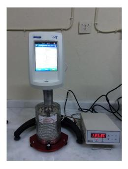
Figure 1. Rotational Viscometer (RV) test device
