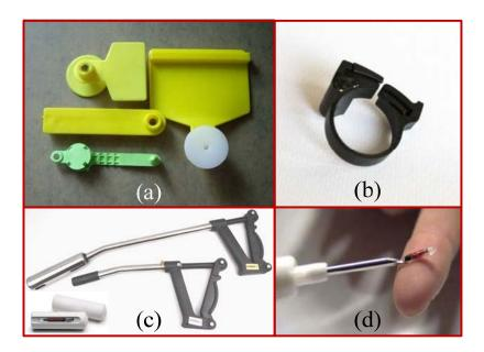
are passive tags used for pets like dogs, cats, fish etc. at LF and HF band. Generally, glass coated tags, smaller than a grain of rice, are injected into animals.
