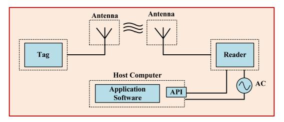
Figure 1. RFID System Components
