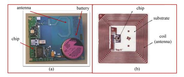
Figure 3. a) Active and b) passive RFID tag
