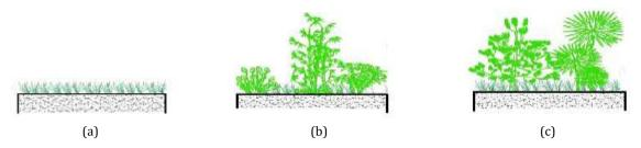
**Figure 3.** a) Superficially planted green roof b) Semi-densely planted green roof c) Densely planted green roof section (Seckin and Seckin, 2016).
