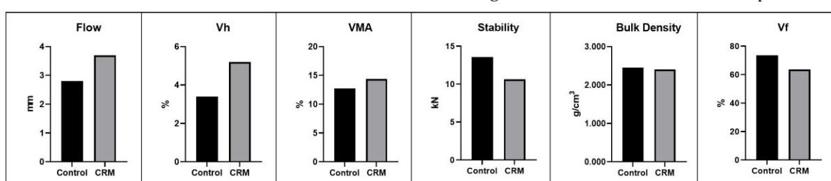
Figure 5. Marshall test results
