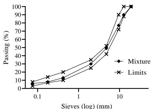
**Figure 1.** Gradation limits for HMA
