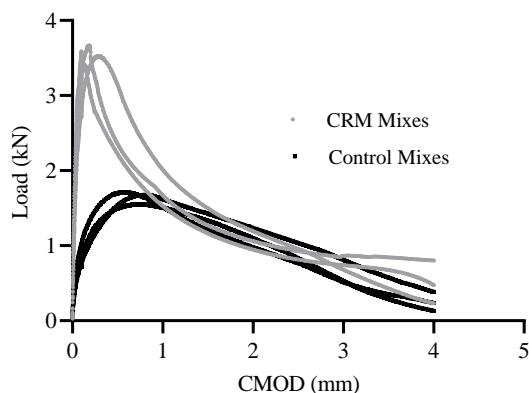
**Figure 7.** The work of fracture plots
