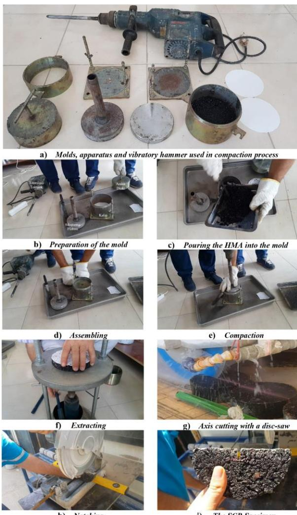
Figure 3. Preparation steps of the SCB specimen
