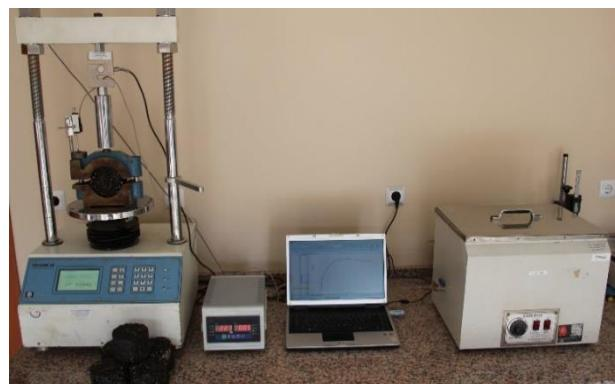
**Figure 2.** VJ Tech - TRISCAN 50 loading device
