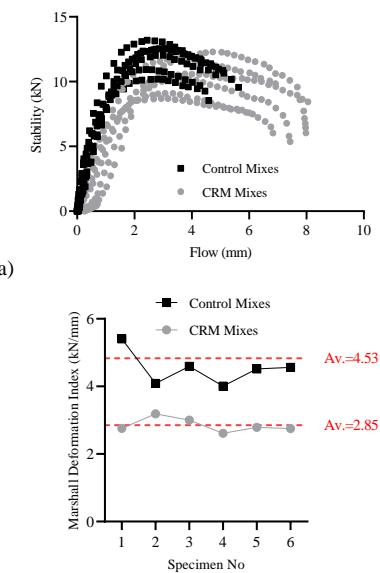
Figure 6. Marshall deformation index in specimens
