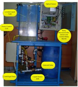
Figure 6. Mechatronic liquid level measurement system
