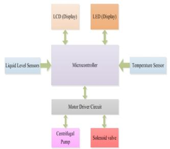
Figure 2. Block diagram of the mechatronic liquid level measurement system
