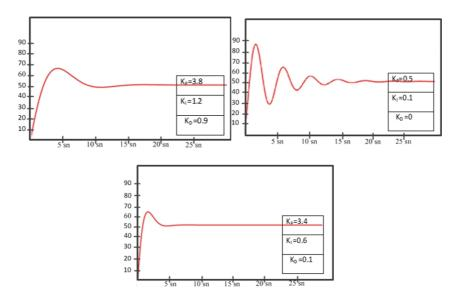
Figure 5. Simulation oscilloscope images for different  $K_{P},\,K_{I}\,and\,K_{D}\,values$
