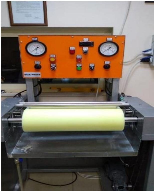
Figure 4. Size press coating machine
