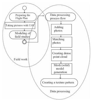
Figure 6. Processes in the UAV photogrammetry method
