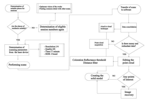
Figure 4. Process flow realized in software
