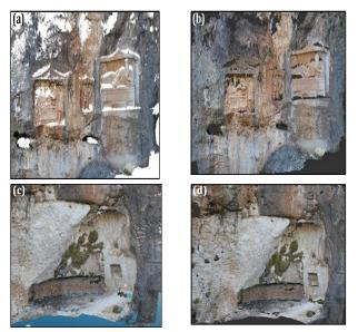
**Figure 5.** (a), (c) Point cloud obtained by TLS method (b), (d) 3D model
