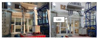
Figure 4 Precast RC beam-column connection shake table tests, [18]
