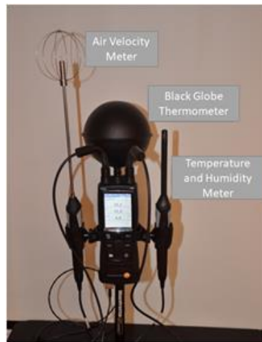
Figure 1. TESTO 480 thermal comfort measurement device
