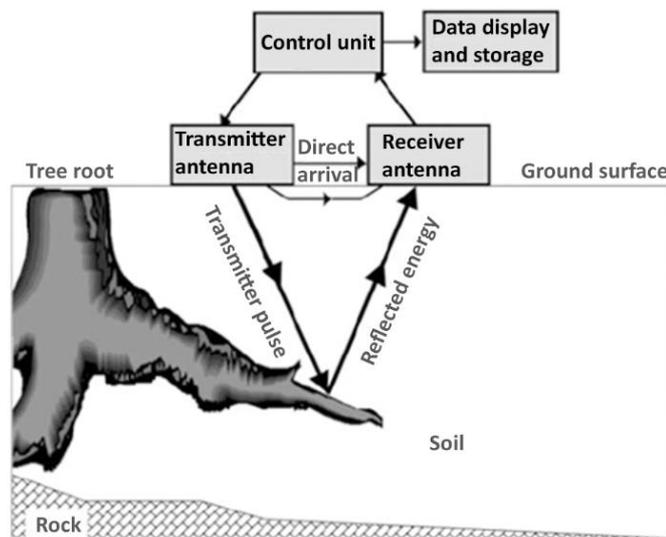
Figure 10. Working principle of GPR (Stover et al., 2007)
