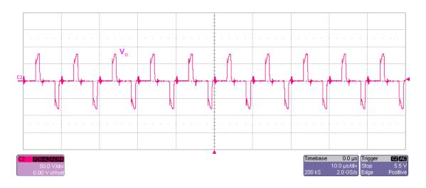
Fig. 6 Bidirectional output voltage measured across the load of proposed MMC with four HB-SMs.
