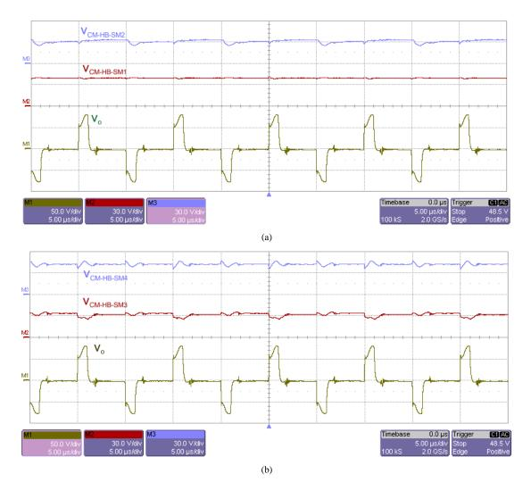
Fig. 7. The capacitor and load voltage waveforms of the built MMC: (a) The load and capacitor voltage of HB-SM1 and HB-SM2, v<sub>CM-HB-SM1</sub> and v<sub>CM-HB-SM2</sub> (b) The load and capacitor voltage of HB-SM3 and HB-SM4, v<sub>CM-HB-SM3</sub> and v<sub>CM-HB-SM4</sub>.
