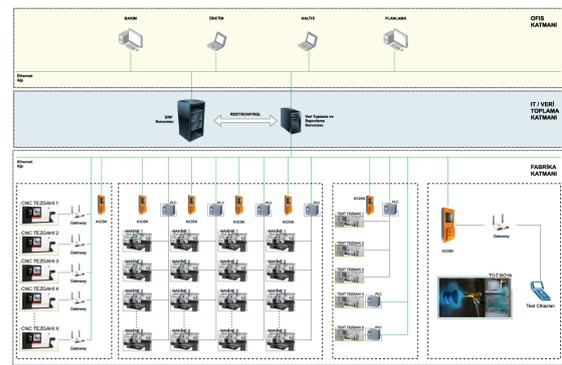
Figure 14. Topology of the digital transformation system.
