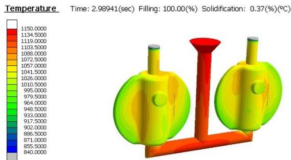
Figure 7. Casting simulation.
