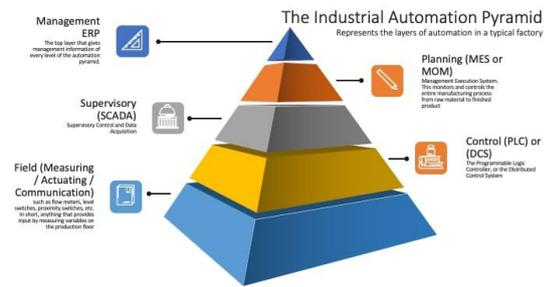
Figure 4. The industrial Automation Pyramid [38].
