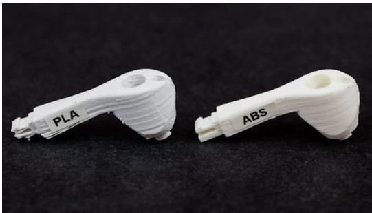
**Figure 2.** 3D printed samples appearance [26].
