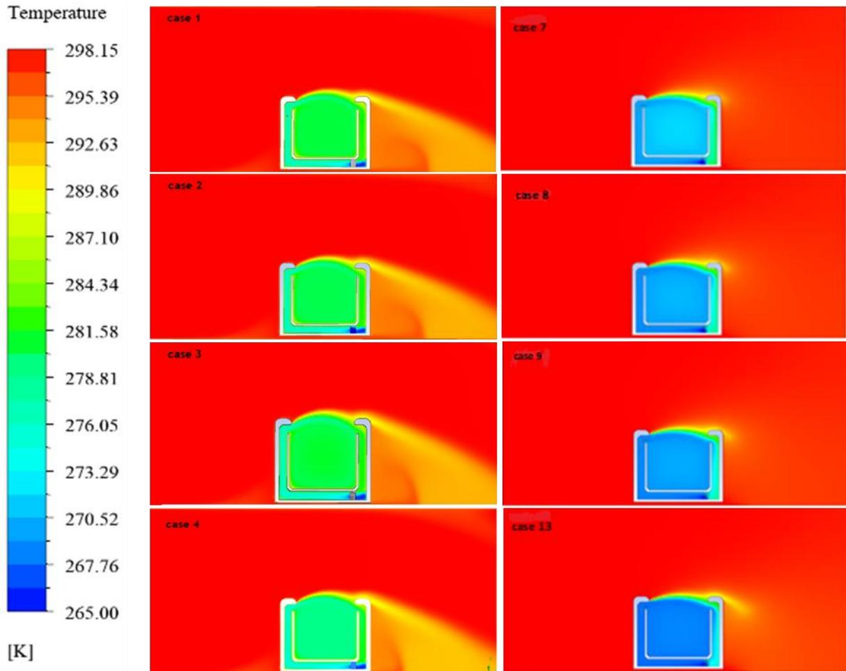
**Figure 3.** Temperature contours for Case 1-4, Case 7-9, and Case 13
