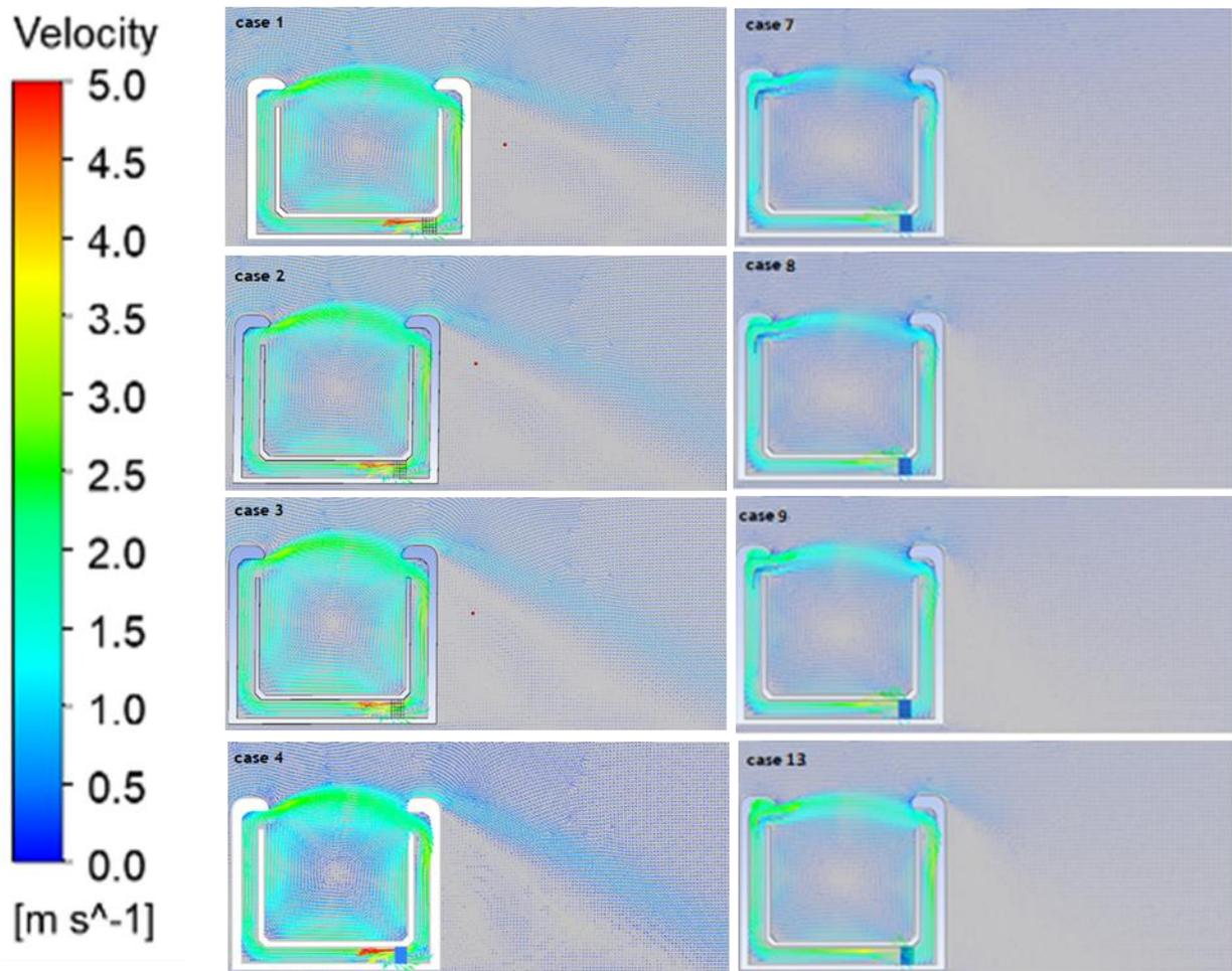
**Figure 4.** Velocity vectors for Case 1-4, Case 7-9, and Case 13
