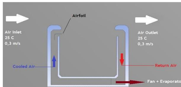
**Figure 1.** Refrigerator Airflow Model
