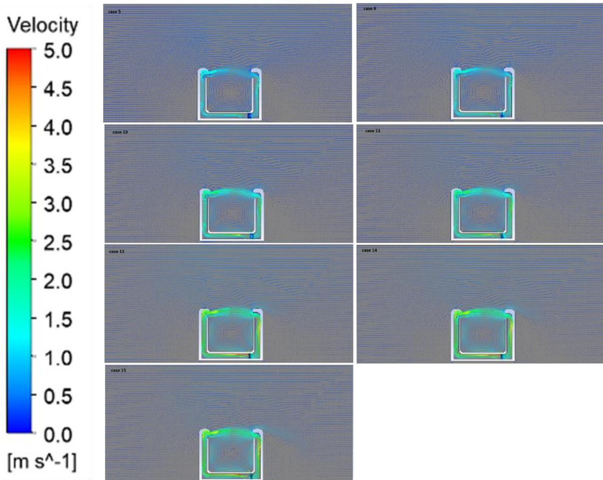
**Figure 6.** Velocity vectors for Case 5-6, Case 10-12, and Case 14-15
