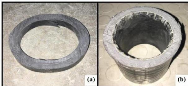
**Figure 7.** Fracture test specimens: (a) after flattening test, (b) after drift-expansion test
